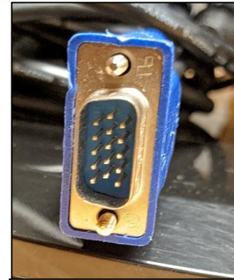
This is a VGA cable, used to carry video only
