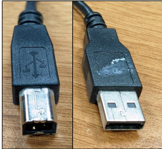
This is a USB cable, used to make your laptop interactive/touch with the panel or board
