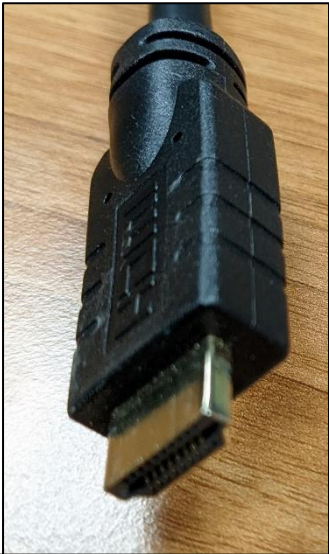
This is a HDMI cable, used to carry video and audio signals (this is the preferred option)
