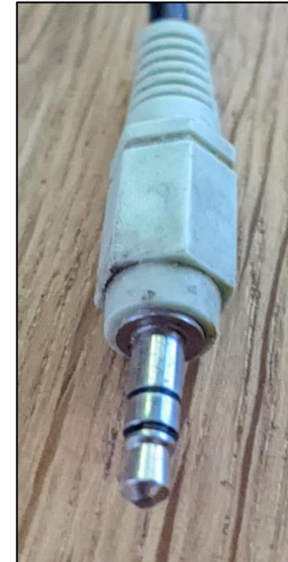
This is an audio cable with a jack plug at each end
